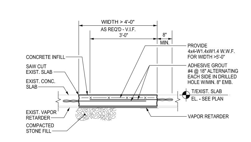
TYPICAL SLAB-ON-GRADE INFILL DETAIL (WIDTH < 4'-0") S-002 SCALE:3/4" = 1'-0"
