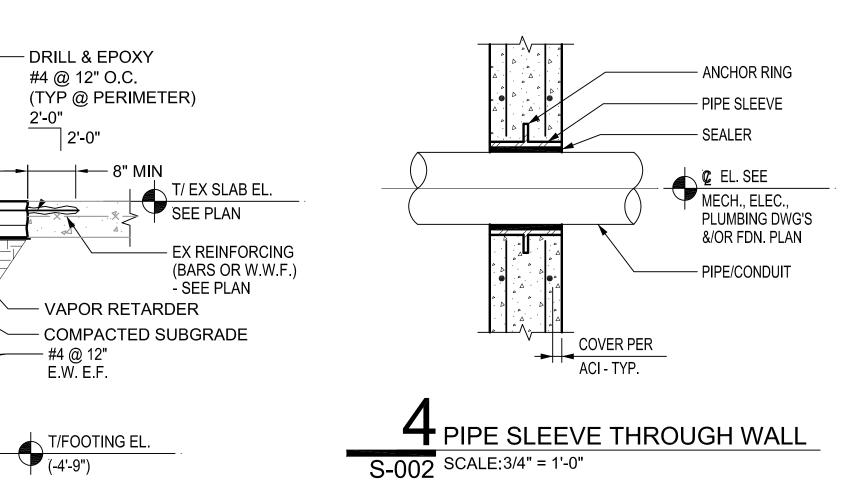
1. SEE ARCHITECTURAL, MECHANICAL AND PLUMBING DRAWINGS FOR SLEEVE DETAILS, SIZE & LOCATIONS.
