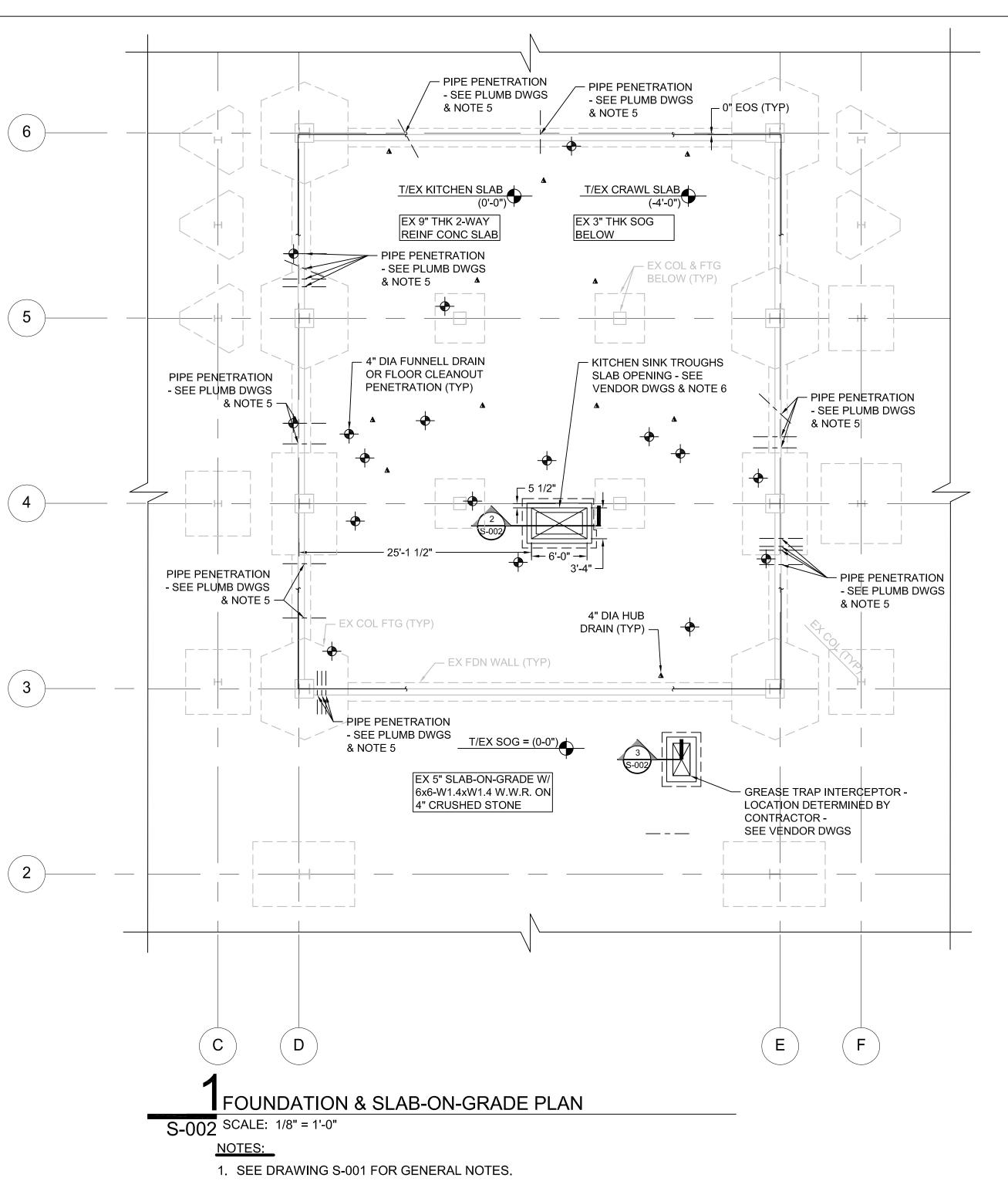
2. TOP OF SLAB ELEVATION 0'-0" ABOVE REFERENCE ELEVATION 301'-0" 3. COORDINATE ALL EMBEDS, PIPE/CONDUIT SLEEVE SIZE AND ELEVATIONS, ETC. WITH INTERIOR, MECHANICAL, ELECTRICAL, PLUMBING DRAWINGS AND CONTRACTORS.
